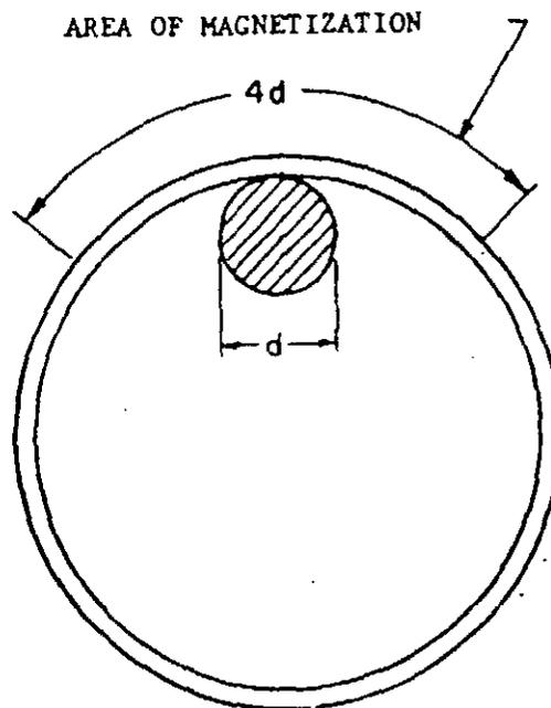
FIGURE 1. Circular magnetization.
