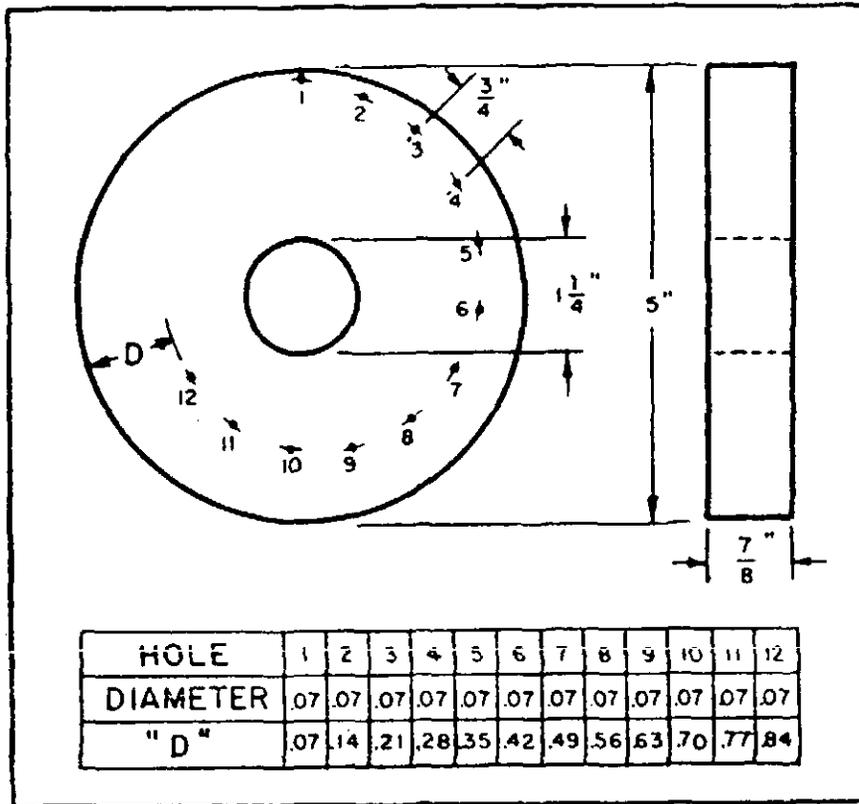
FIGURE 2. Ring specimen with artificial sub-surface discontinuities.
